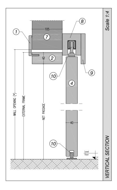
(\*) WALL OPENING TO BE CONSIDERED AS INTERNAL SUB-FRAME OR DRYWALL OPENING
